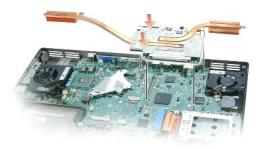
2. Tighten the four captive screws on the video card/thermal cooling assembly.
