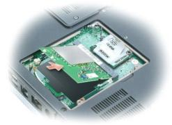
2. Connect the antenna cables to the Mini PCI card.
