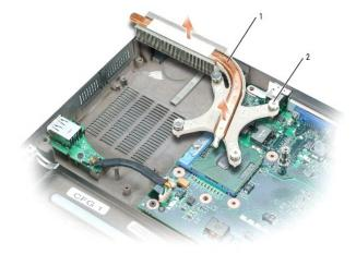
microprocessor thermal-cooling assembly
